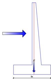
$$\begin{aligned} \text{Berat volume tanah, } \gamma &= 1,535 \text{ T/m}^3 \\ \text{Sudut gesek dalam, } \phi &= 7^\circ \\ \text{Kohesi, } c &= 0,184 \text{ kg/cm}^2 = 18,442 \text{ kpa} \\ \text{Gaya total, } \Sigma P &= 18,9515 \text{ T} \end{aligned}$$
